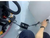
has undervoltage protection function, when the machine voltage is less than 21V, it will automatically cut off the power, and prohibit to use the equipment, then you need to charge in time, and continue to use.
